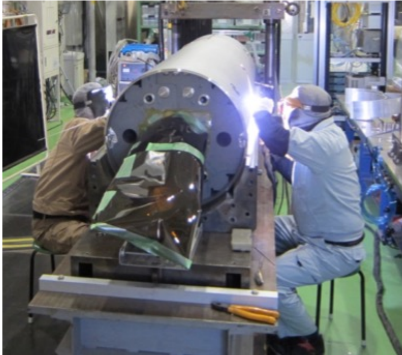
Figure 1: D1 test magnet being assembled.
