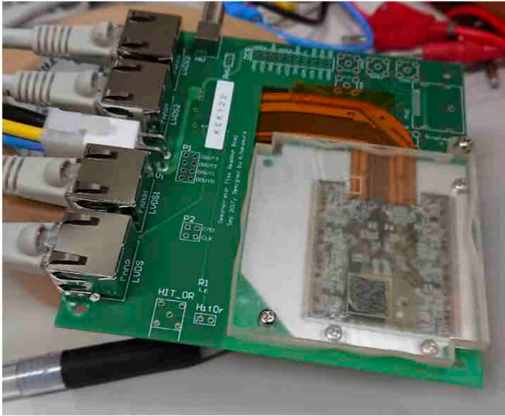
Figure 6: A test system for the prototype pixel detector.
