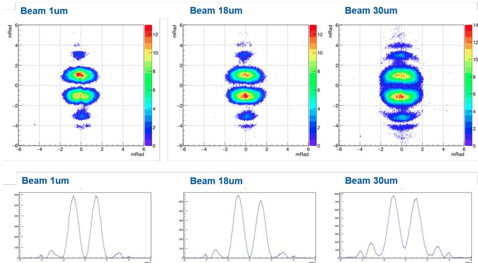
Fig. 6: First Diffraction Radiation images for different beam sizes.
