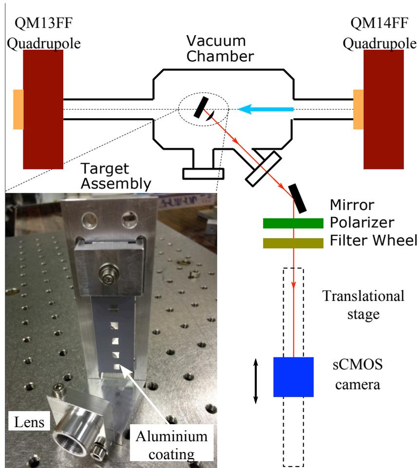
Fig. 1: OTR optical line scheme with target picture
