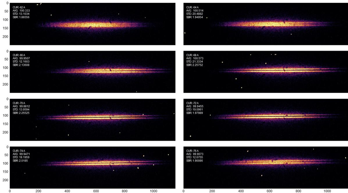
Fig. 2: Images of the vertical polarization of the OTR signal at different strengths of the QM14FF quadrupole
