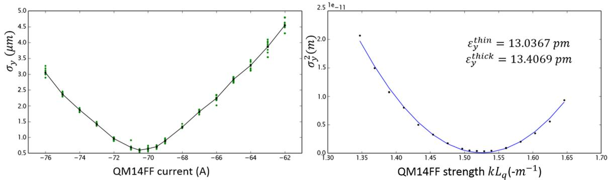
Fig. 4: Results of the beam size measurements as function of the quadrupole current (left), squared beam size as function of the quadrupole strength and fitted emittance (right).
