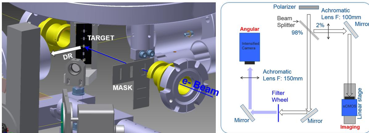
Fig. 5: Diffraction Radiation monitor instrument details: in vacuum set-up (left) and optical line (right).
