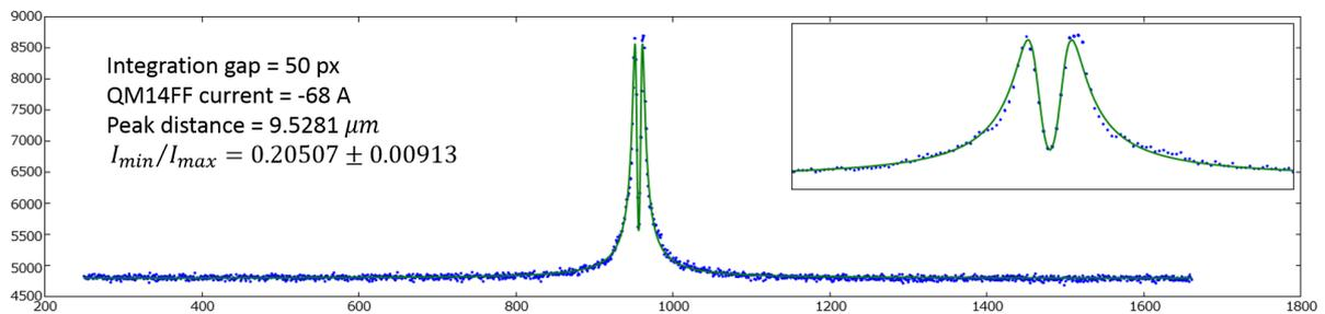
Fig. 3: Example of OTR vertical projection. Data point (blue) obtained by integrating 50 pixel around the center of mass of the image. The parameters of the distribution are obtained from the fit.
