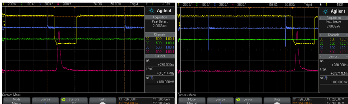
Fig. 3: IP-BSM photon detector signals for the 1 st bunch (left) and 2 nd bunch (right). The detector gate, beam and photon signals are shown in yellow, blue and pink, respectively.
